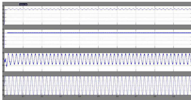
Fig.14 shows the simulation waveforms of boost voltage V_{dc} , PV voltage V_{pv} , grid current I_g , grid voltage V_g under 50% of rated condition
